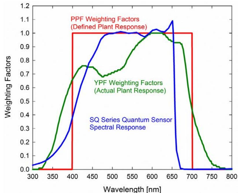
Radiation weighting factors for PPFD (defined plant response to radiation), YFPD (measured plant response to radiation), and Apogee SQ Series quantum sensors (sensor sensitivity to different wavelengths of radiation).
